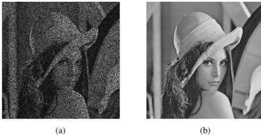
Fig.1.1(a) Image (with dimension 512 \times 512 ) captured using PCI sensing matrix with 50% sampling ratio and with zeros filled at positions not sampled (b) Image reconstructed from subsampled image using 'db4' wavelet
