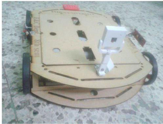
IOT Robot Structure
