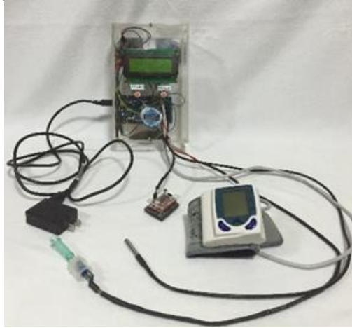
Figure 8: The prototype of vital signs checking system
