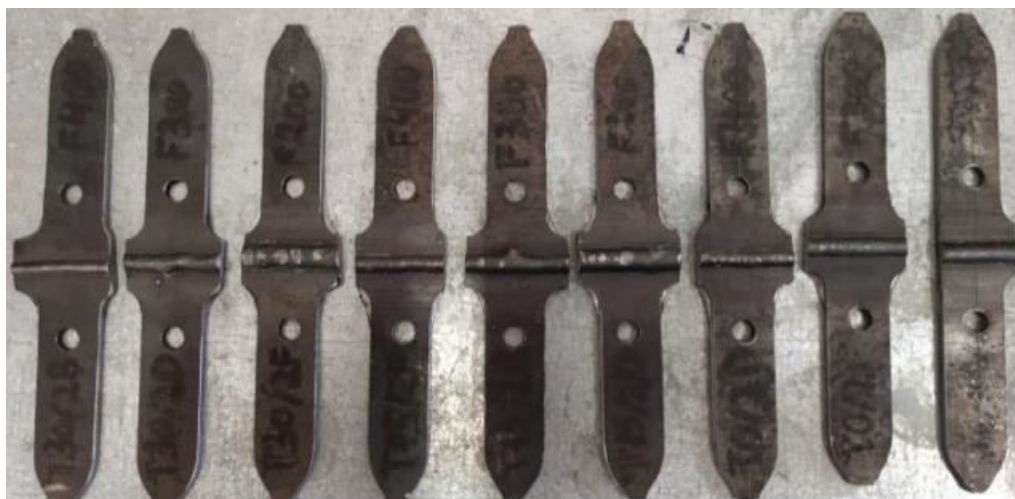
Figure 4: Weld samples for macrography inspection
