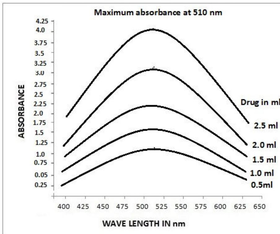
**Fig. 2: Absorption spectrum of Tamsulosin-Phenol red complex**
