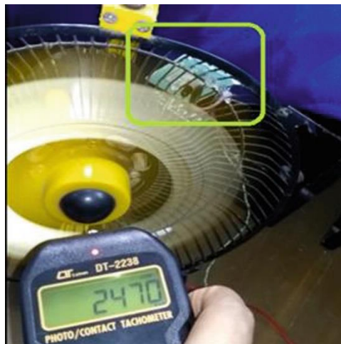
Fig 2-3 Measurement of the speed of BLDC using a digital tachometer
