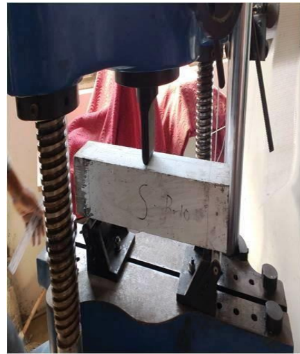
Fig 3.5: Testing of Beam Specimens on UTM
