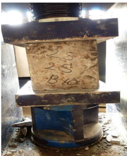
Fig 3.4: Testing of Cube Specimens on CTM
