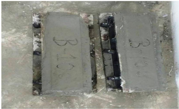
Fig3.2: Casted Beam Specimens
