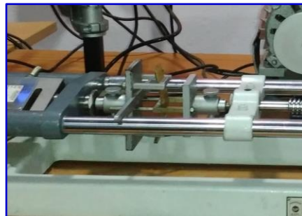
Fig 4.2: Composite under flexural test
