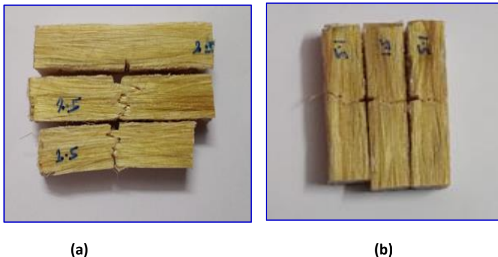
Fig 4.5 (a): NaOH treated Neem fiber (b) Without NaOH treated Neem fiber epoxy composites
