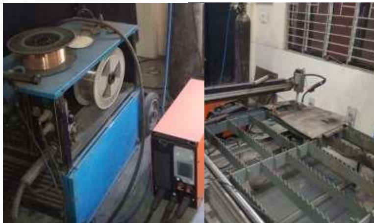
Figure : Wire feed Mechanism Figure : Robotic WAAM platform
