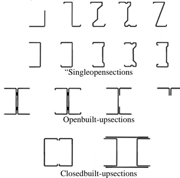
**Figure-1.** Typical forms of sections for cold-formed members [10].”
