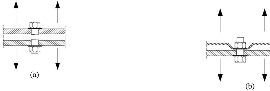
Figure-4.Failure modes of bolted connections in tension [7].
