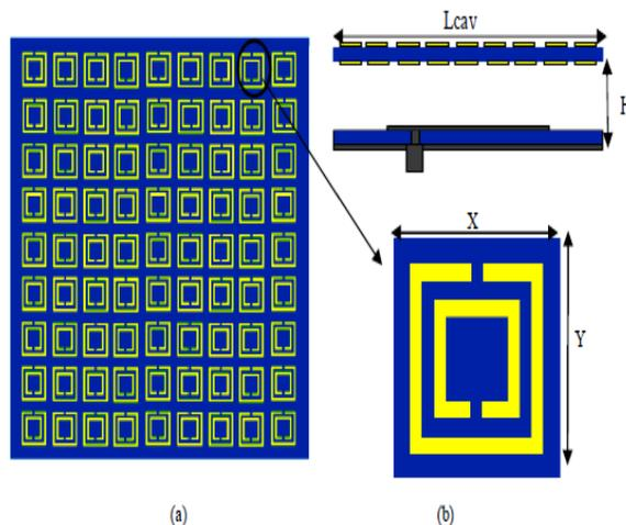
**Fig. 1.** Patch antenna with a double layer MMT layer. (a) top and and front view of the antenna (b)SRR unit cell.
