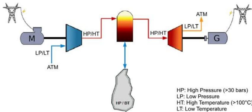
Figure 1. Storing energy in compressed adiabatic air (Source: EDF)
