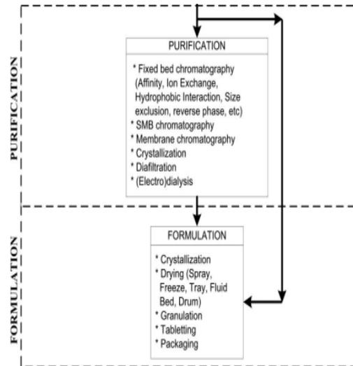
**Figure 1. Generalized block diagram of downstream processing.**
