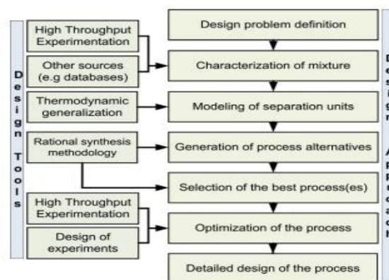
Figure 2. A hybrid approach to bioseparation process design.
