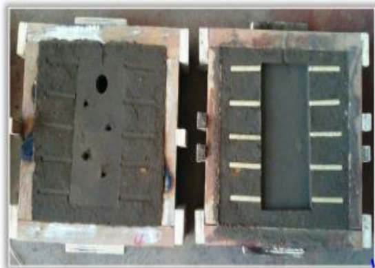
Figure 1: Sand mould with chills
