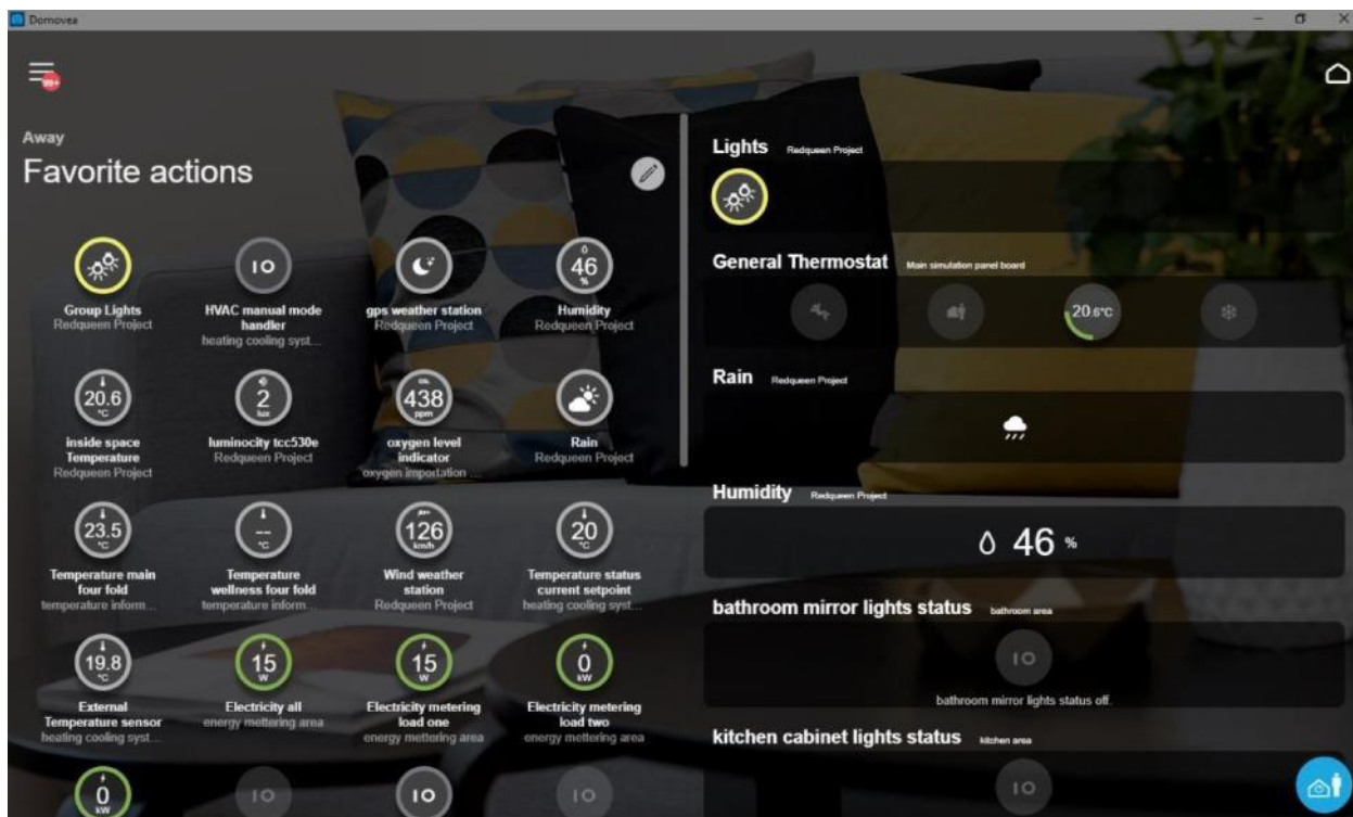
Figure 10: Domovea Expert IOT server Smart Thermostat and Peripheral Data Points Dashboard
