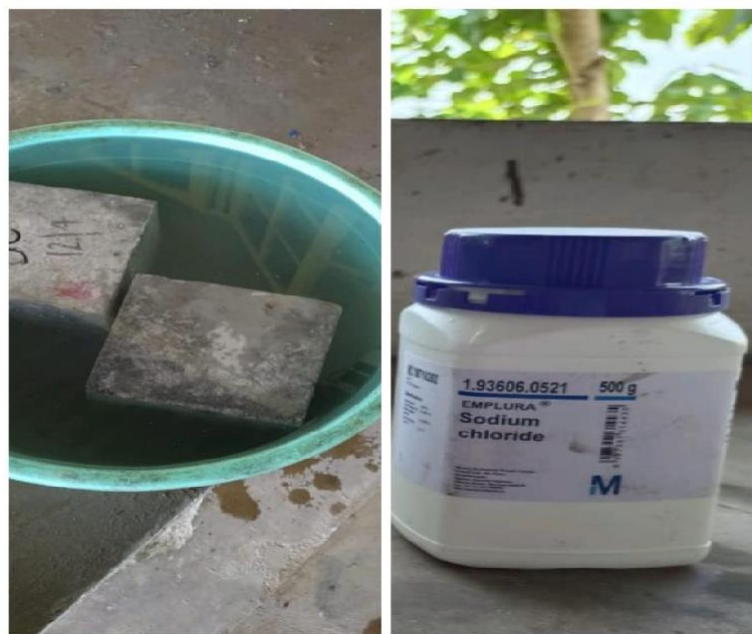
Fig 5.4.3: Chloride Penetration Test
