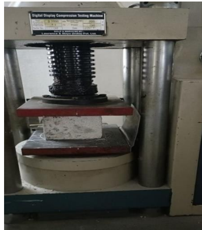
Fig 5.2: Compressive strength test for cement cube
