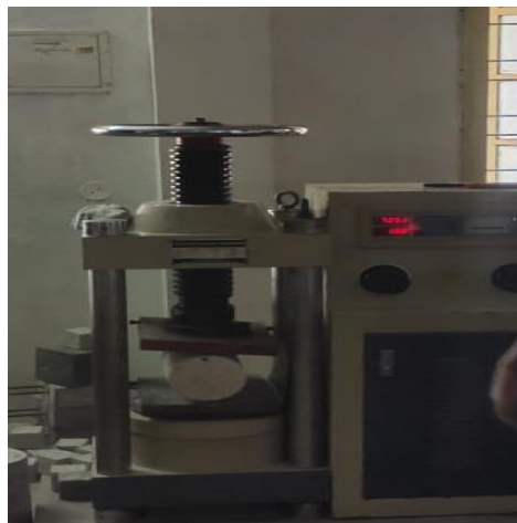
Figure 5.2 Split tensile strength testing
