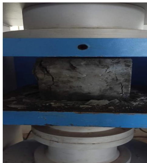
Fig 5.8: compression of cubes
