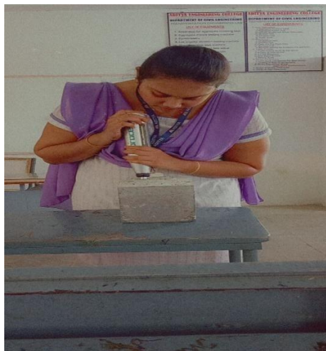
Fig 5.12 rebound hammer test
