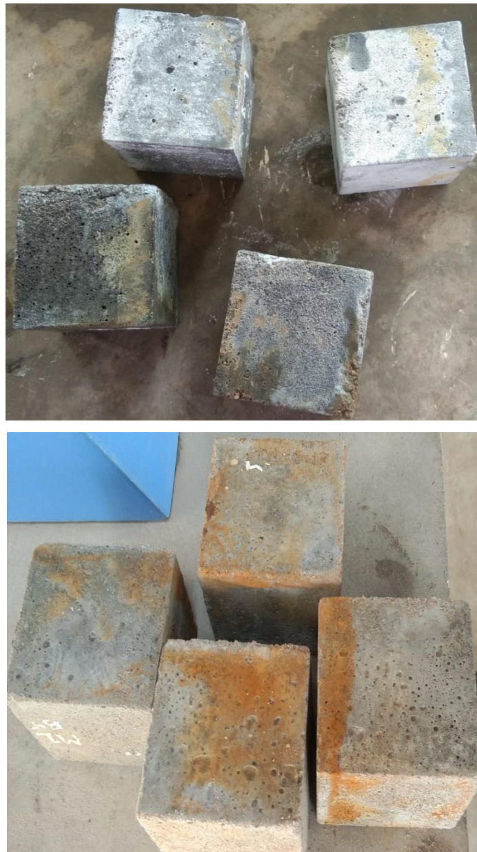
Fig 4.4 Acid curing specimens
