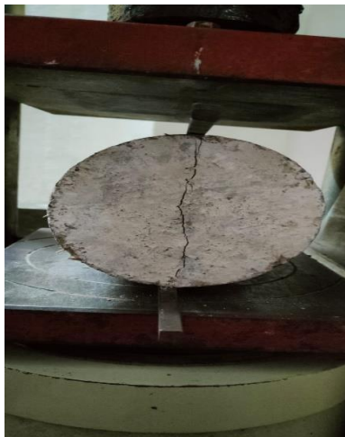
Figure 4.2: Split tensile strength testing
