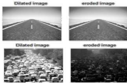
Fig. 8 Dilated and eroded images of reference and traffic.
