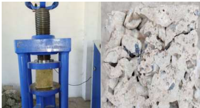
Fig 5.5 Testing of cube specimen
