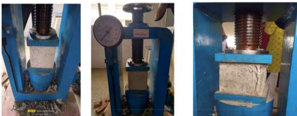
Fig. 7: Compressive strength test for cubes.
