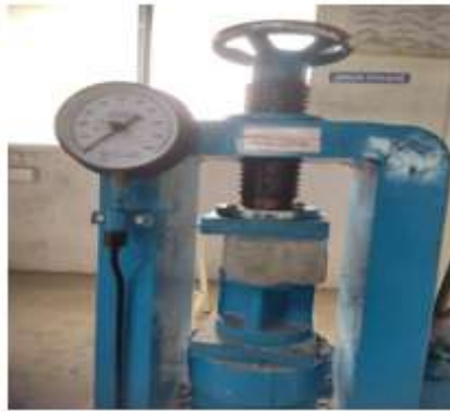
Fig. 7: Testing of paver block specimen.
