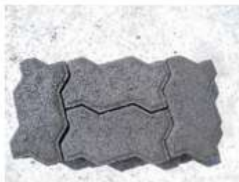
Fig. 8: No Efflorescence present on Paver block.
