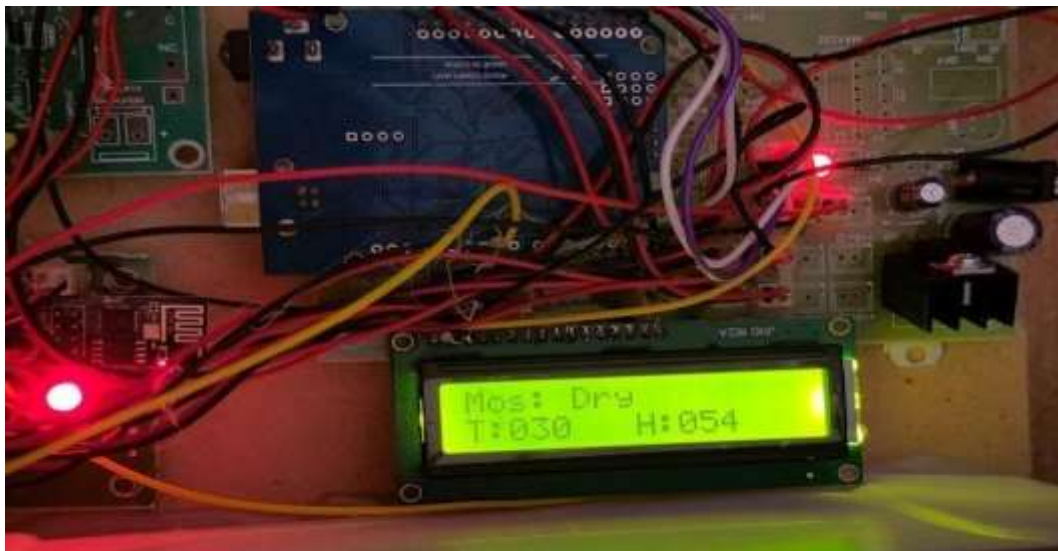
Figure 4 Lcd indicating the soil is dry
