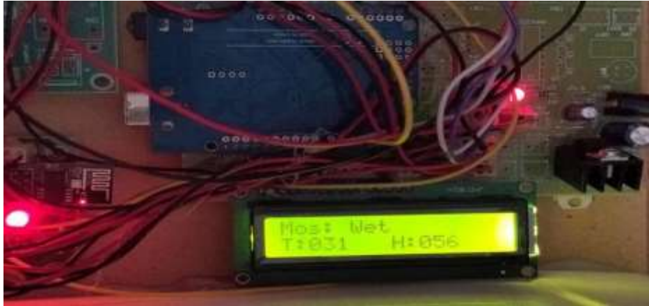
Figure 5 Lcd indicating the soil is wet
