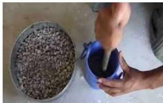
Fig. 4 Aggregate impact value test in progress.
