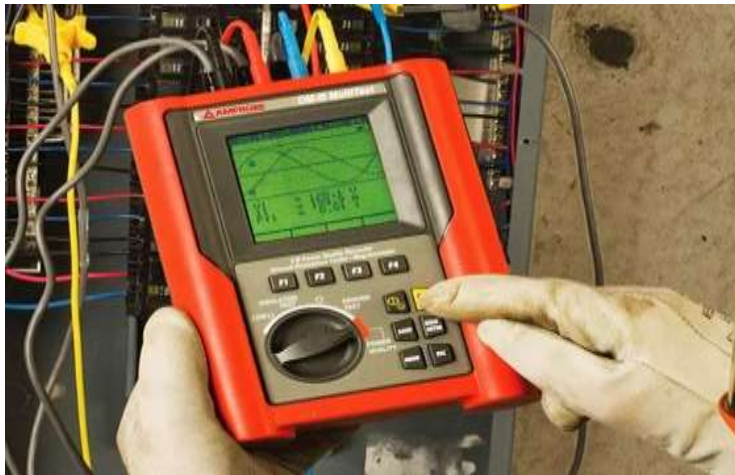
Figure 5 Power Quality Measuring Instrument ( Network Stabilizer)
