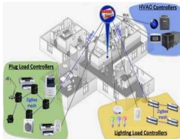
Fig. 1. BEMOSS system architecture for commercial buildings
