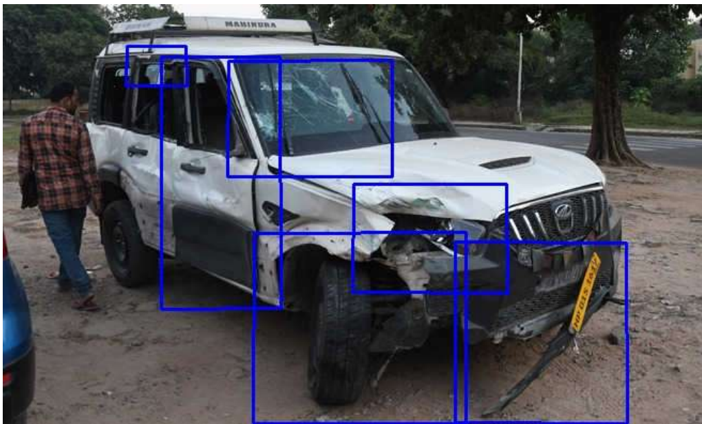
Figure 3 Single Car Damage Detection
